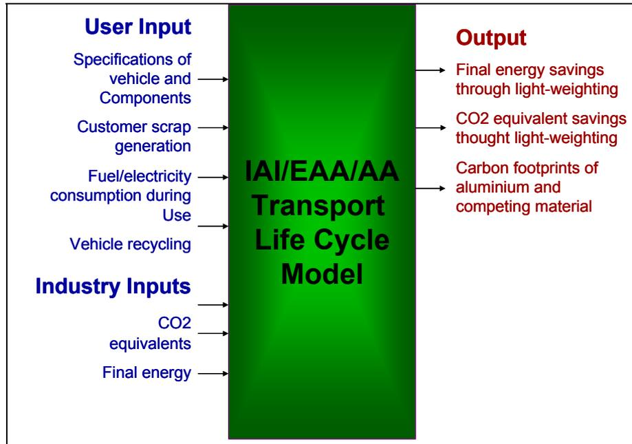
Figure 3: Inputs to and outputs from the aluminium in transport life cycle model
