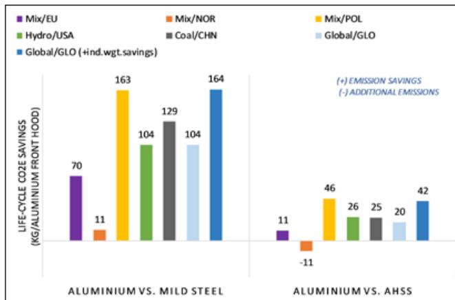
Figure 4: Total lifecycle CO<sub>2</sub>e savings for an aluminum front hood used in a battery electric vehicle taxi compared to a mild steel or an AHSS front hood. A 35% indirect weight savings can be applied to visualize GHG savings from downsizing of the vehicle components.
