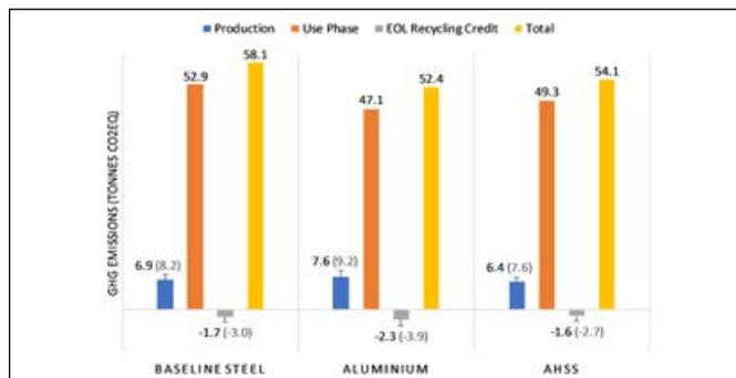
Figure 2: Lifecycle CO<sub>2</sub>e emissions by stage comparing a mild steel, aluminum, and AHSS BIW for a family car with a gasoline internal combustion engine. Error bars and values in brackets represent the results with zero percent recycled metal content.
